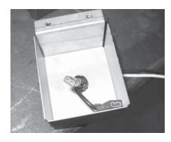
13) Connect the female ends of the red and white wires to the thermodisc.
